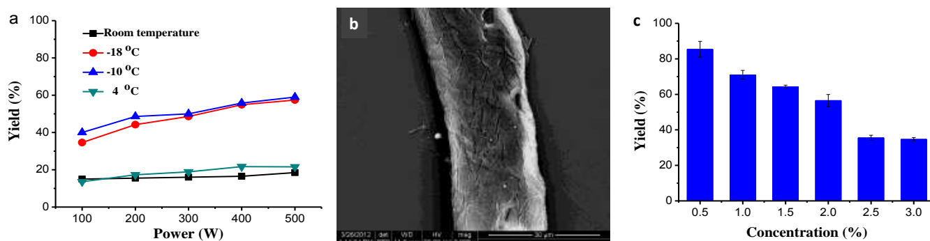
Fig. 6. (a) Effects of pre-cool temperature and ultrasonic energy on NFs yields, when the ultrasonic time was set at 30 min (1 s pause every 2 s sonication), and the cellulose concentration was 2%; (b) SEM image of ultrasonication treated cellulose; (c) Effects of cellulose concentration on NFs yield, when the pre-cool temperature was -10 °C, the ultrasonic energy was 500 W, and the ultrasonic time was 30 min.
